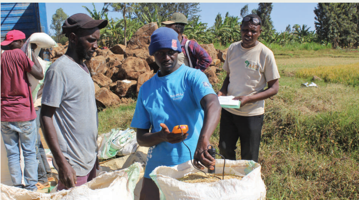
Mr. James Munene, a field officer, ICOSEED, measuring moisture content after hybrid rice harvest in Kirinyaga County, Kenya.
